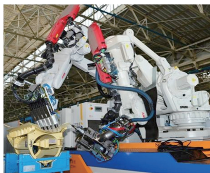
图7 机器人自动测量-铣削系统集成应用 Fig.7 Integration application of robot automatic measuring-milling system
